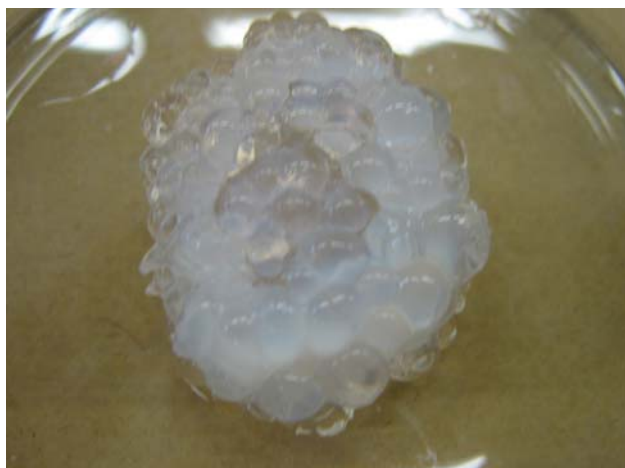
Fig. 10 White skin layer and bubbles characteristic of all hydrogels, after deswelling at 60 °C for 1 h
